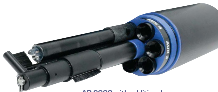
AP-6000 with additional sensors removed exposing central cleaning shaft
